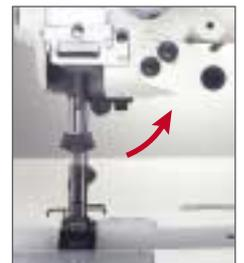
**Bottom-feed micro-adjustment mechanism is provided as standard. (LU-1510N-7, LU-1511N-7)**
